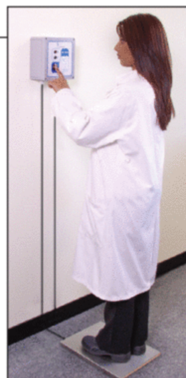
FIGURE 4. If static-dissipative footwear is specified, it can also be tested for ongoing effectiveness using test stations that test the ground leakage from the individual, via the footwear, to ground. These devices help prevent incorrect shoes from being used in static-sensitive environments
